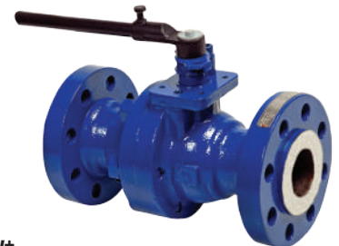
Flow+ 2-Piece Carbon Steel Ball Valve ZR6 • 2"–6": Class 600, flanged • WCB or LCC body, regular port • ISO mounting pad
