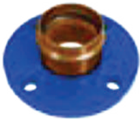
NIBCO Copper Companion Flange PC641 • 2½"–4": 200 PSI CWP • P x Flange
