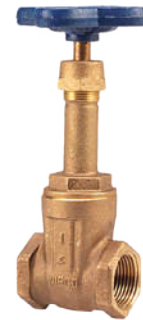
NIBCO Class 125 Bronze Gate Valve T/S-111 • ¼"–3": 200 PSI CWP • Threaded (NPT) or soldered • Rising stem • Screwed-in bonnet
