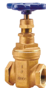
NIBCO Class 150 Bronze Gate Valve T-133 • ¼"–3": 300 PSI CWP • Threaded (NPT) • Non-rising stem • Screwed-in bonnet
