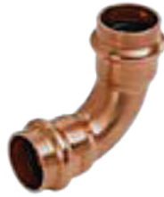
NIBCO Copper 90° Elbow PC607 • ½"–4": 200 PSI CWP • P x P
