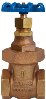
NCI Class 300 Bronze Gate Valve GTVB-TBZ3333U • ¼"–2": 1000 PSI CWP • Threaded (NPT) or soldered • Rising stem • Union bonnet CRN
