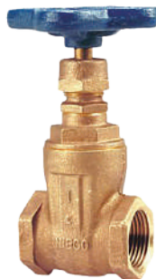
NIBCO Class 125 Bronze Gate Valve T/S-113 • ¼"–3": 200 PSI CWP • Threaded (NPT) or soldered • Non-rising stem • Screwed-in bonnet
