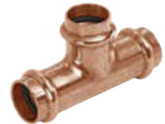
NIBCO Copper Tee PC611 • ½"–4": 200 PSI CWP • P x P x F
