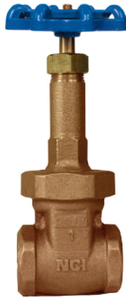
NCI Class 150 Bronze Gate Valve GTVA-(T/S)BZ2333U • 3/8"–2": 300 PSI CWP • Threaded (NPT) or soldered • Rising stem • Union bonnet CRN
