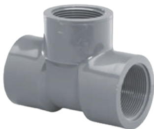
LESSO PVC Sch80 Tee 805 Series • Size: 1/4"-4" • FIPT x FIPT x FIPT
