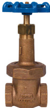
NCI Class 300 Bronze Gate Valve GTVA-TBZ3333U • ¼"–2": 1000 PSI CWP • Threaded (NPT) or soldered • Rising stem • Union bonnet CRN
