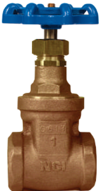
NCI Class 150 Bronze Gate Valve GTVB-(T/S)BZ2333 • ¼"–3": 300 PSI CWP • Threaded (NPT) or soldered • Non-rising stem • Union bonnet CRN
