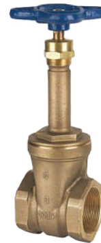
NIBCO Class 150 Bronze Gate Valve T-131 • ¼"–3": 300 PSI CWP • Threaded (NPT) • Rising stem • Screwed-in bonnet
