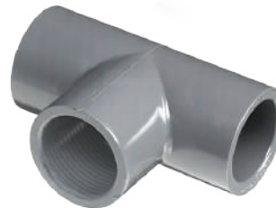
LESSO PVC Sch80 Tee 802 Series • Size: 1/2"-2" • SOC x SOC x FIPT
