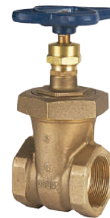
NIBCO Class 150 Bronze Gate Valve T/S-136 • ¼"–3": 300 PSI CWP • Threaded (NPT) or soldered • Non-Rising stem • Union bonnet
