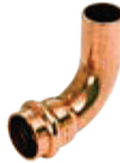
NIBCO Copper 90° Elbow PC607-2 • ½"–4": 200 PSI CWP • FP x P
