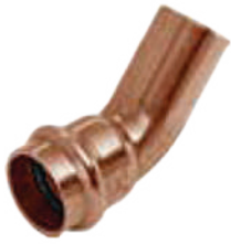
NIBCO Copper 45° Elbow PC606-2 • ½"–4": 200 PSI CWP • Ftg x P
