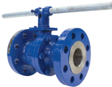
Flow+ 2-Piece Carbon Steel Ball Valve ZF3 • 2"–8": Class 300, flanged • WCB or LCC body, full port • ISO mounting pad
