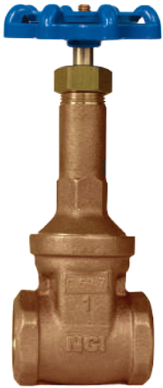
NCI Class 150 Bronze Gate Valve GTVA-(T/S)BZ2333 • ¼"–3": 300 PSI CWP • Threaded (NPT) or soldered • Rising stem • Screwed-in bonnet CRN
