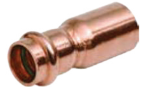
NIBCO Copper Reducer PC600-2 • ½"–4": 200 PSI CWP • Ftg x P
