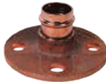
NIBCO Copper Companion Flange PC741 • 1"–2": 200 PSI CWP • P x Flange
